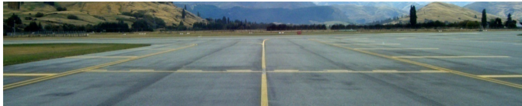
16-4 - Runway Hold Point Marking – Alpha 3
